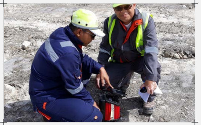
RemScan being used in situ on the lagoon sediments.
